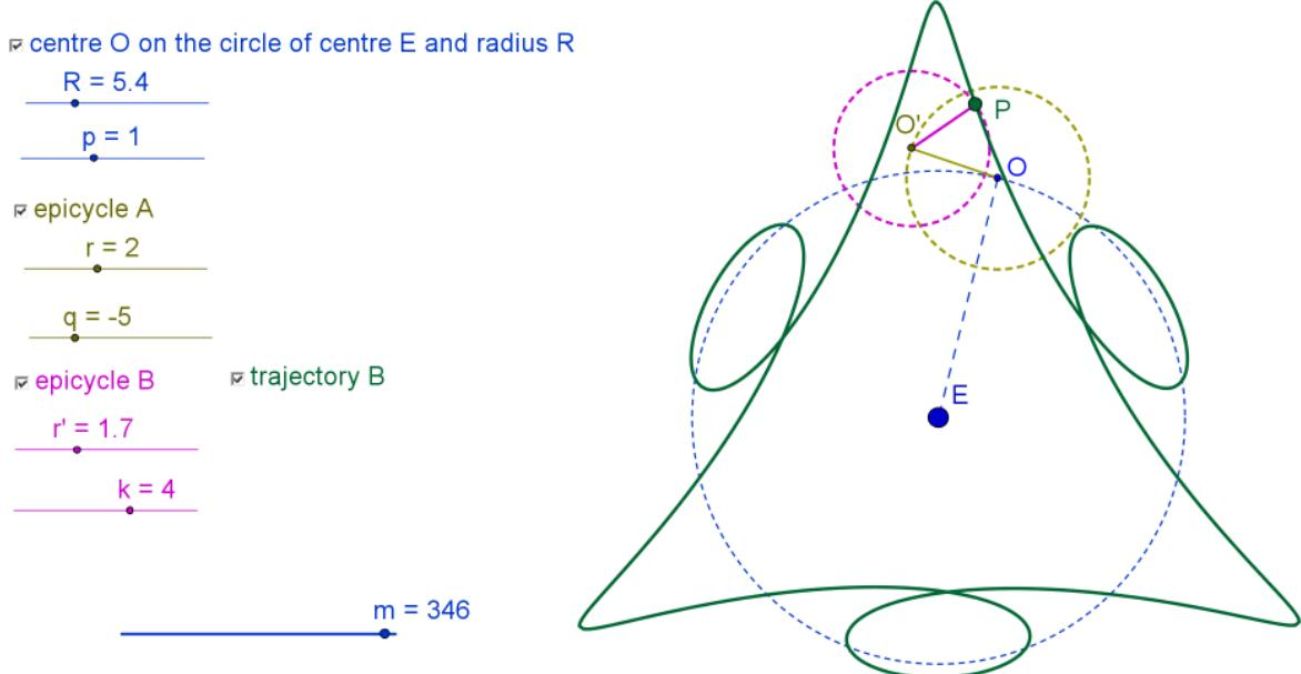
On this example, during the time O turns once anticlockwise around E, O' turns five times clockwise around O and P four times anticlockwise around O' but you can try a lot of other combinations!
